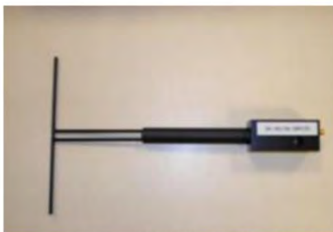
Figure 1 – Satimo COMOSAR Validation Dipole
