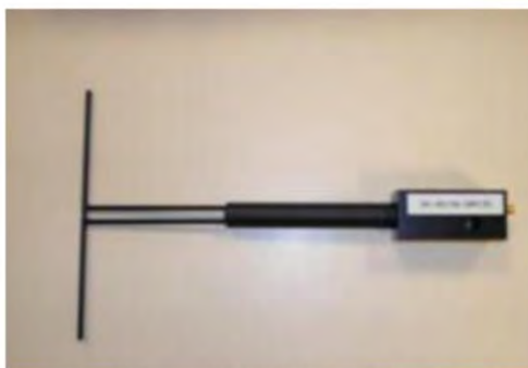
Figure 1 – Satimo COMOSAR Validation Dipole
