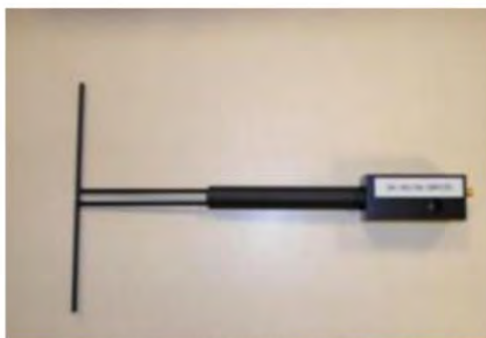
Figure 1 – Satimo COMOSAR Validation Dipole
