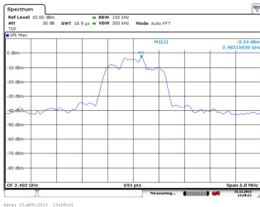
Fig. 31 Conducted Spurious Emission (8DPSK, Ch0, 2.402GHz)
