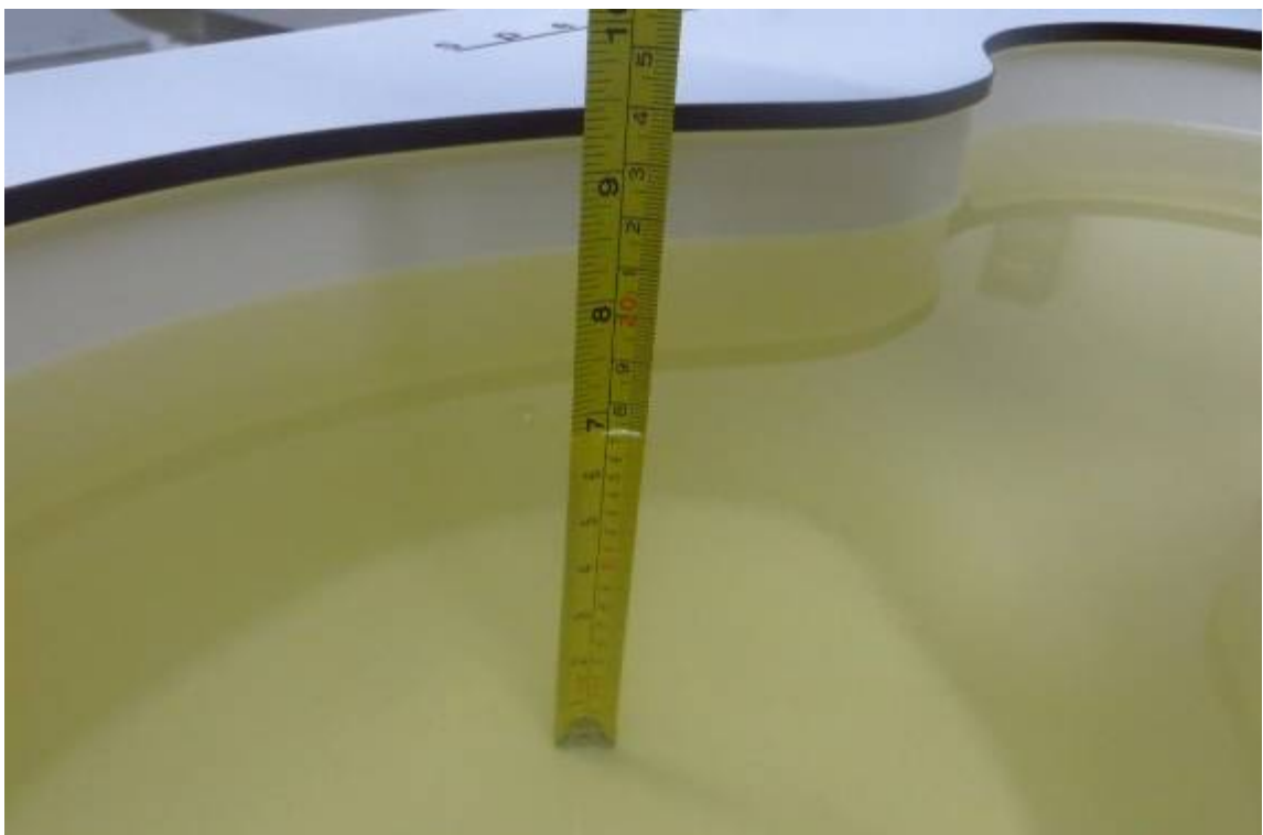
Picture 7-2: Liquid depth in the Flat Phantom (835 MHz) (depth=17.6cm)
