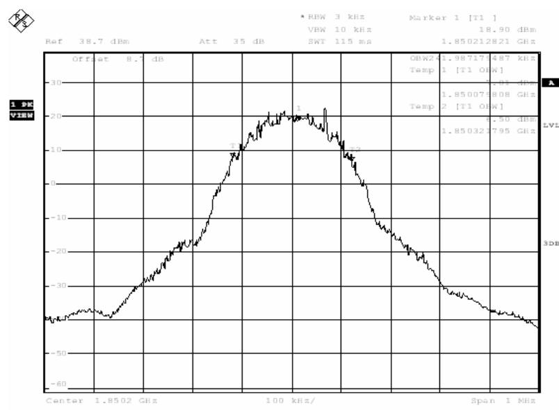
**Channel 661-Occupied Bandwidth**
