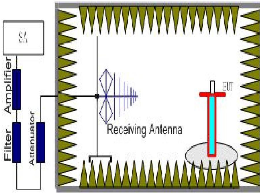
2. The EUT is then put into continuously transmitting mode at its maximum power level during the test. And the maximum value of the receiver should be recorded as (Pr).
