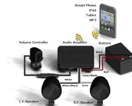
Figure 3. Wiring diagram for BT-900 system. Please note that the wiring plan is the same for both Bluetooth and 3.5mm cable users.
