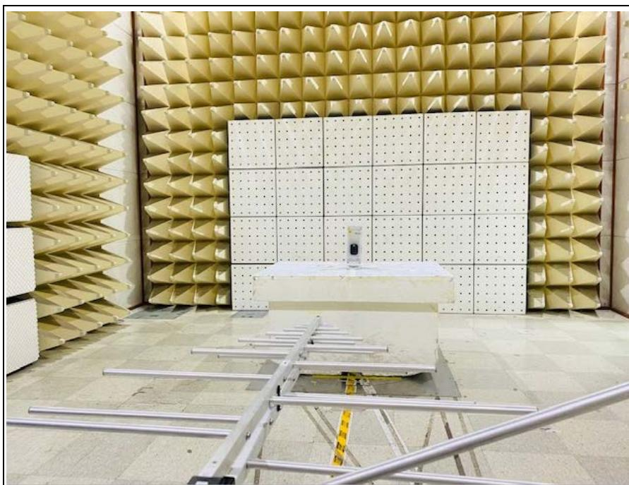
**3. Photo of Radiated Spurious Emission Test (Above 1 GHz)**
