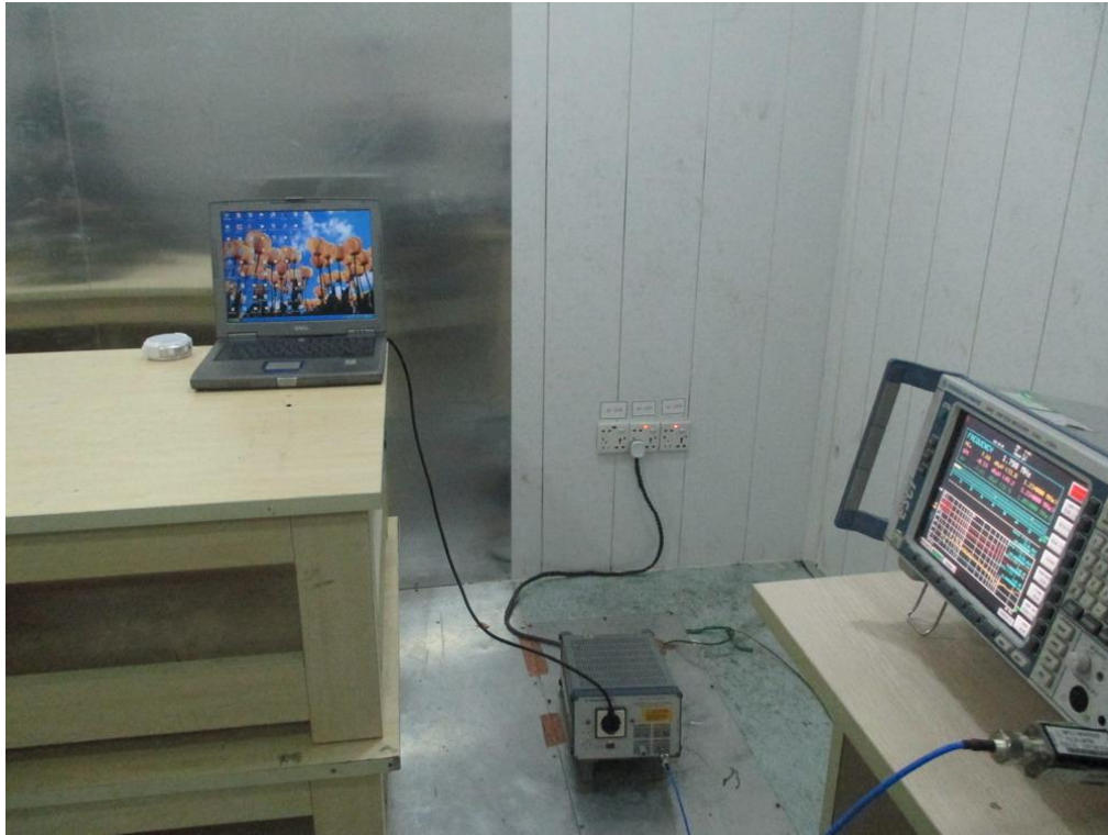
FCC RADIATED EMISSION TEST SETUP
