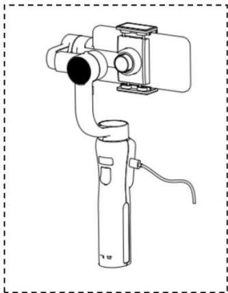
Connect the Micro USB Port on the side of gimbal's handle to a power source SUCH AS a power pack (not include) to extend run-times.
