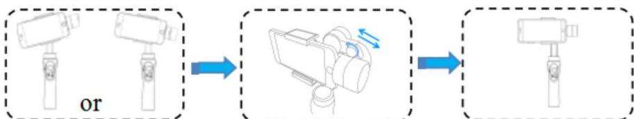
**NOTE:** Proper adjustment of balance ensures better power saving during operation. The gimbal may still function well when the gravity center is not properly configured; however, it may lead to more power consumption on the motors, and can greatly affect the torque output.
