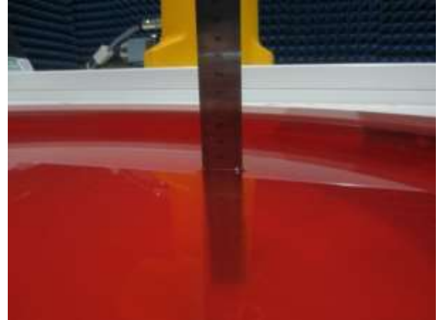
Fig. 9.2 Photo of Liquid Height for Body SAR of ELI V5.0 (850MHz) (depth>15cm)
