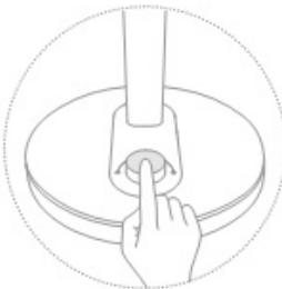
Press the rotating switch to turn the lamp on and off
