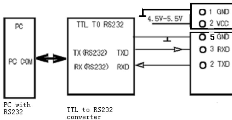
**Note:** As EZ50B mode TTL interface module, so the PC must be added to connect the TTL to RS232 converter, and converter must supply DC 5V of electricity.
