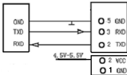
**Note:** EZ50B did not have sleep in the state, the module of the SLE feet must be vacant. In the sleep state when the module must be low, the module can send and receive data.
