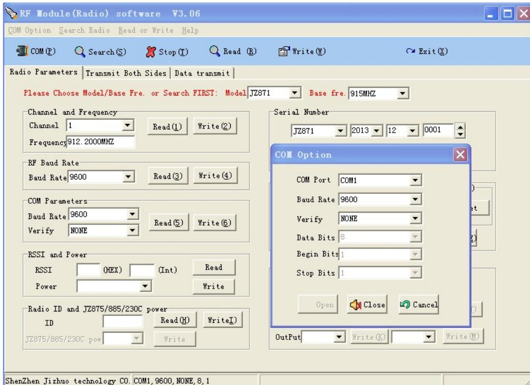
**A、EZ50B module connected to the PC and plug in the power, select the serial port used.**
