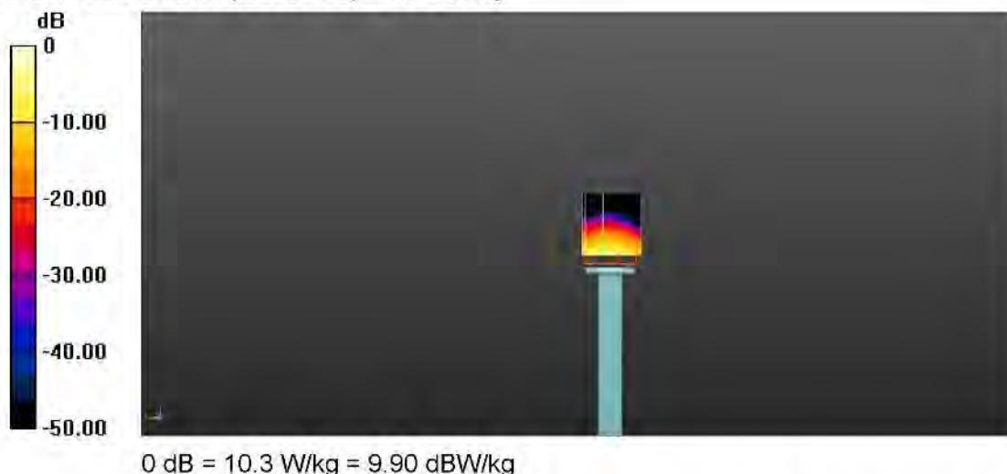
**Dipole validation measurement for Body Tissue/Pin= 100mW ,dist=10mm,f=5800**
