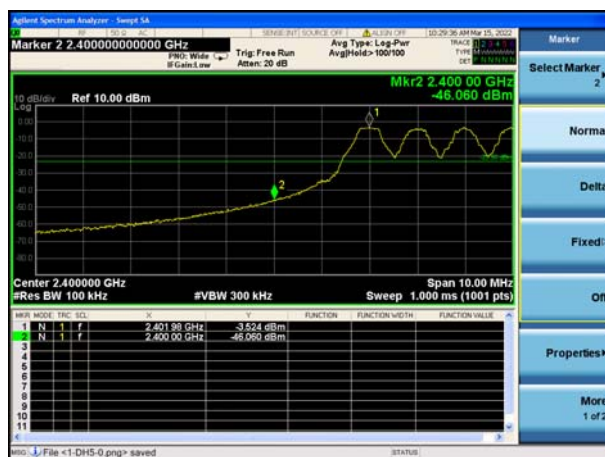
Left Band edge hopping on
