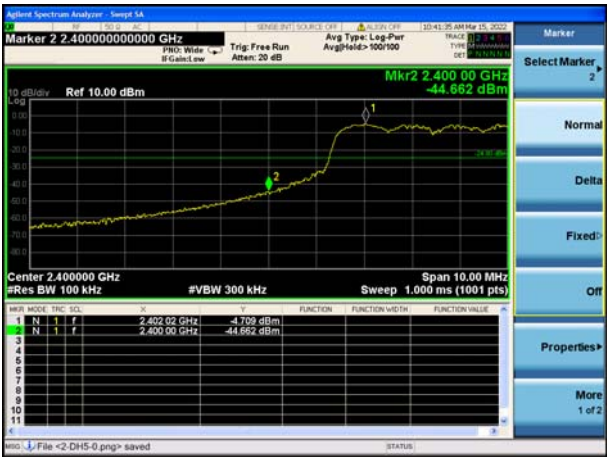
Left Band edge hopping on
