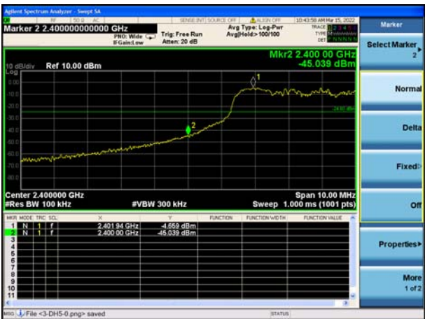
Left Band edge hopping on
