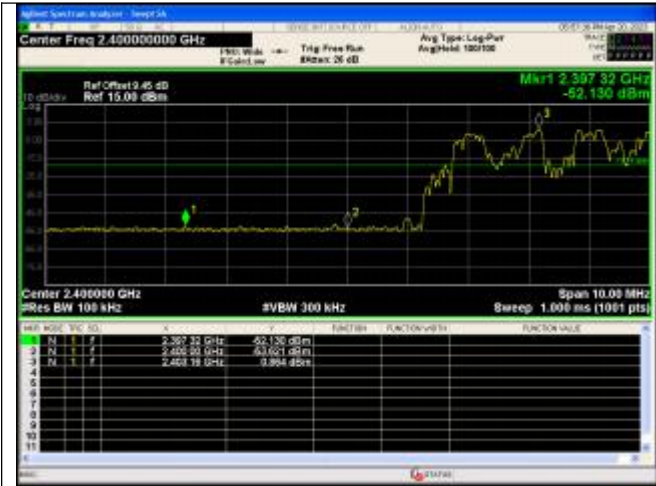
Out Of Band Emission(Left) 8DPSK_3-DH5_Channel Hopping
