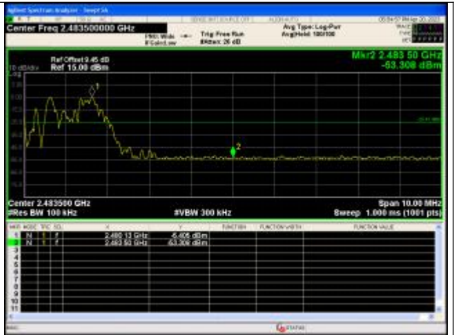
Out Of Band Emission(Right) \pi/4 DQPSK_2-DH5_Channel Hopping
