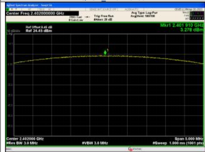
Peak Output Power 8DPSK_Channel 0
