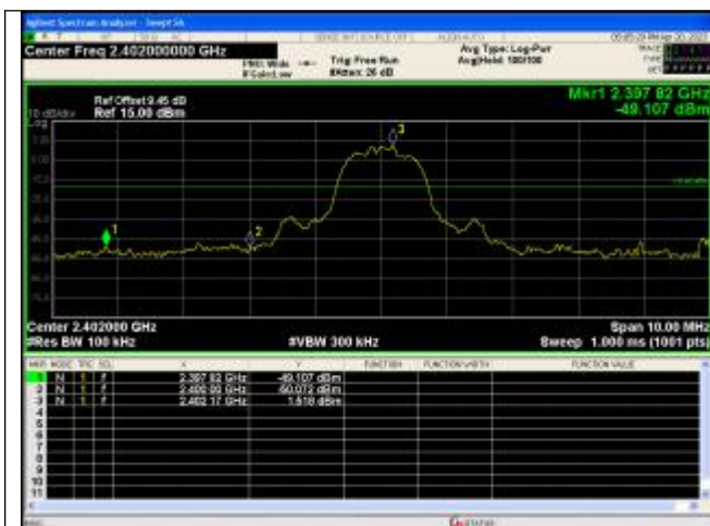
Out Of Band Emission 8DPSK_3-DH5_Channel 0
