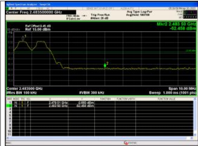
Out Of Band Emission(Right) GFSK_DH5_Channel Hopping
