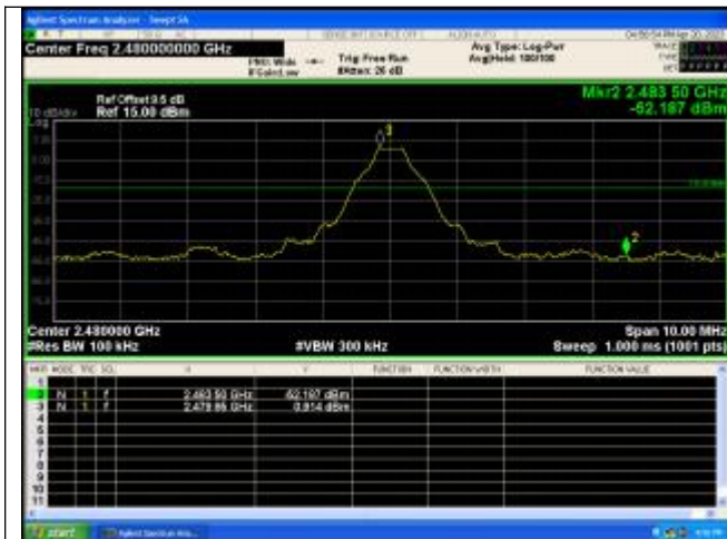
Out Of Band Emission GFSK_DH5_Channel 78
