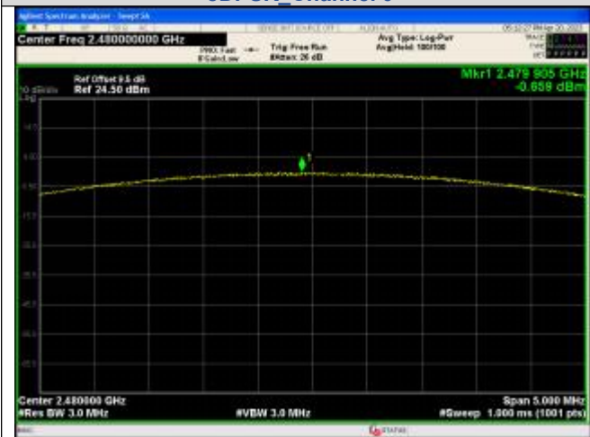
Peak Output Power 8DPSK_Channel 78
