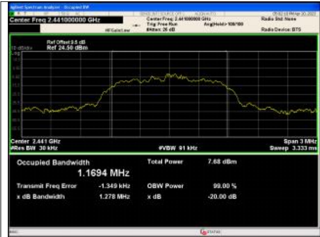
\pi/4 DQPSK 2-DH5 Channel 39
