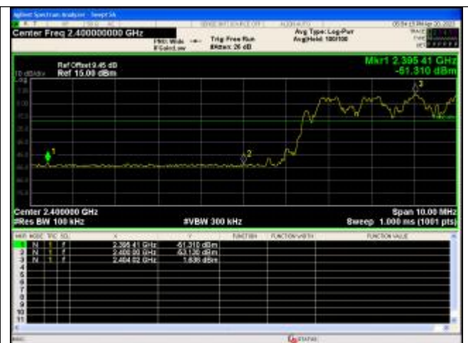
Out Of Band Emission(Left) \pi/4 DQPSK_2-DH5_Channel Hopping
