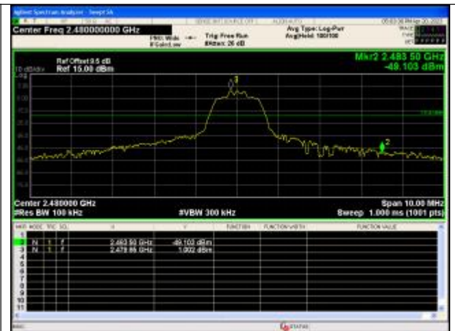
Out Of Band Emission \pi/4 DQPSK_2-DH5_Channel 78
