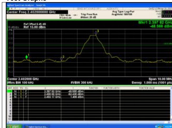
Out Of Band Emission GFSK_DH5_Channel 0
