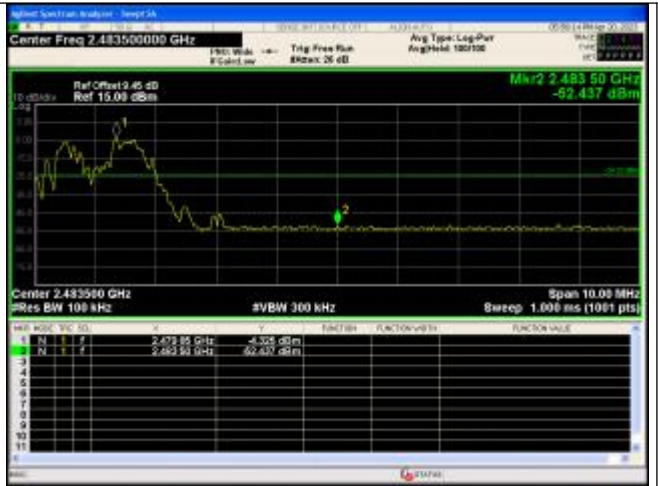
Out Of Band Emission(Right) 8DPSK_3-DH5_Channel Hopping
