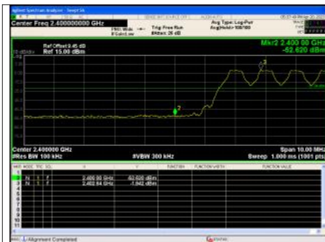
Out Of Band Emission(Left) GFSK_DH5_Channel Hopping
