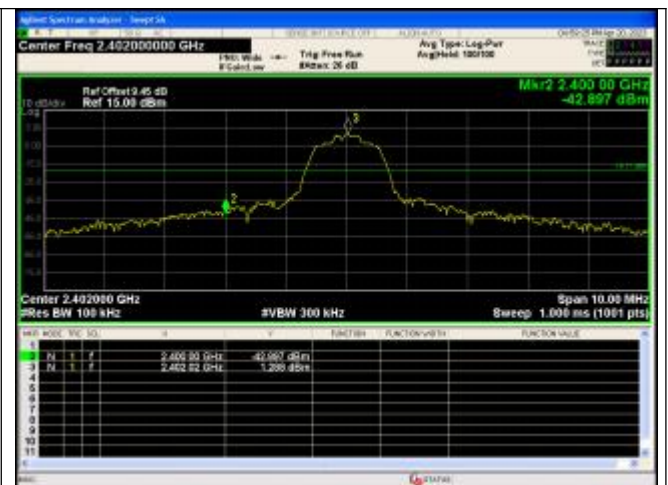
Out Of Band Emission \pi/4 DQPSK_2-DH5_Channel 0
