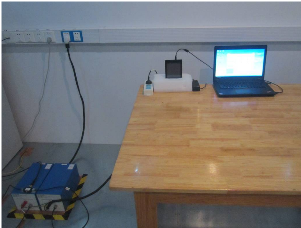
Conducted Emissions Test Setup Front View
