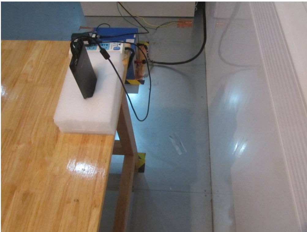
Conducted Emissions Test Setup Side View
