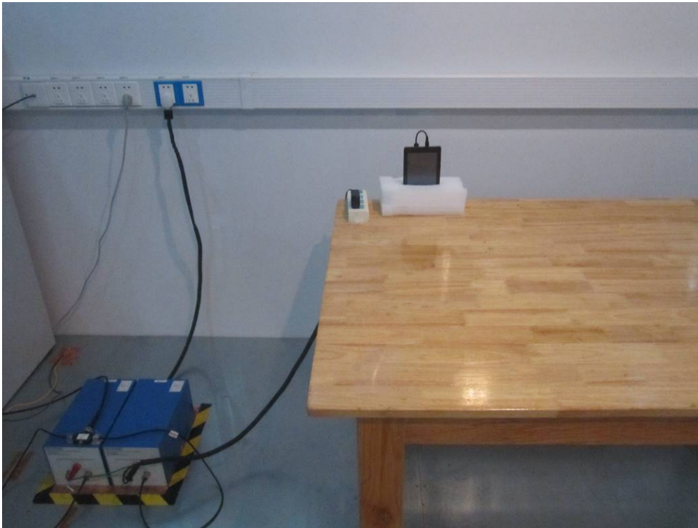
Conducted Emissions Test Setup Front View
