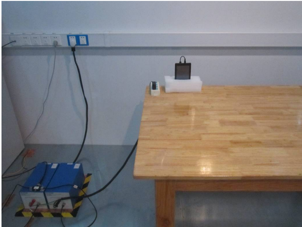
Conducted Emissions Test Setup Front View
