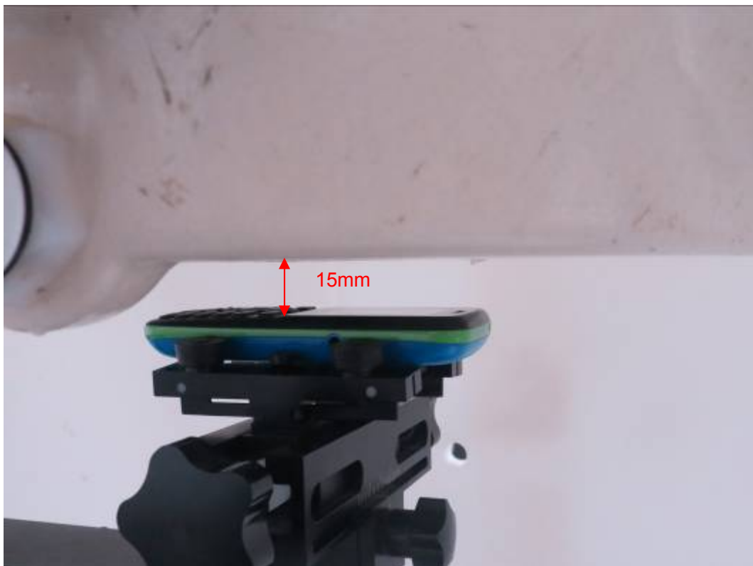
Picture 12: Front Side, the distance from handset to the bottom of the Phantom is 15mm
