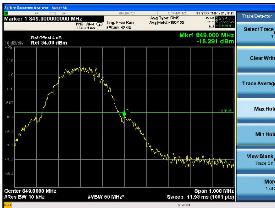
Higher Band Edge Plot on Channel 251
