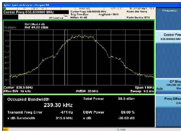
Occupied Bandwidth Plot on Channel 251
