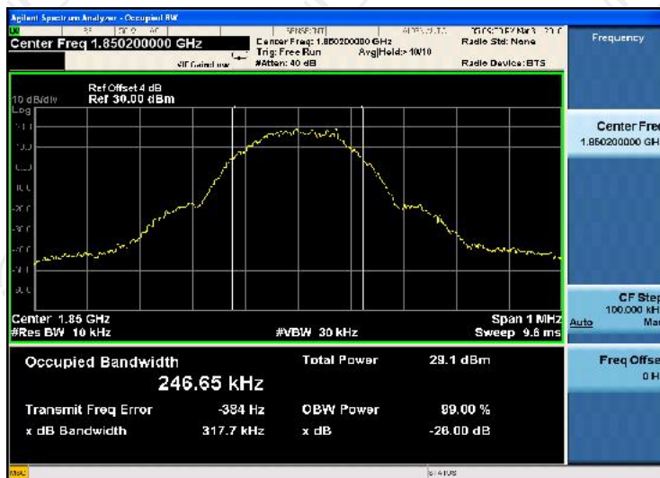
Occupied Bandwidth Plot on Channel 661
