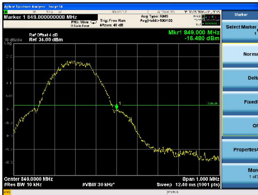
Higher Band Edge Plot on Channel 251
