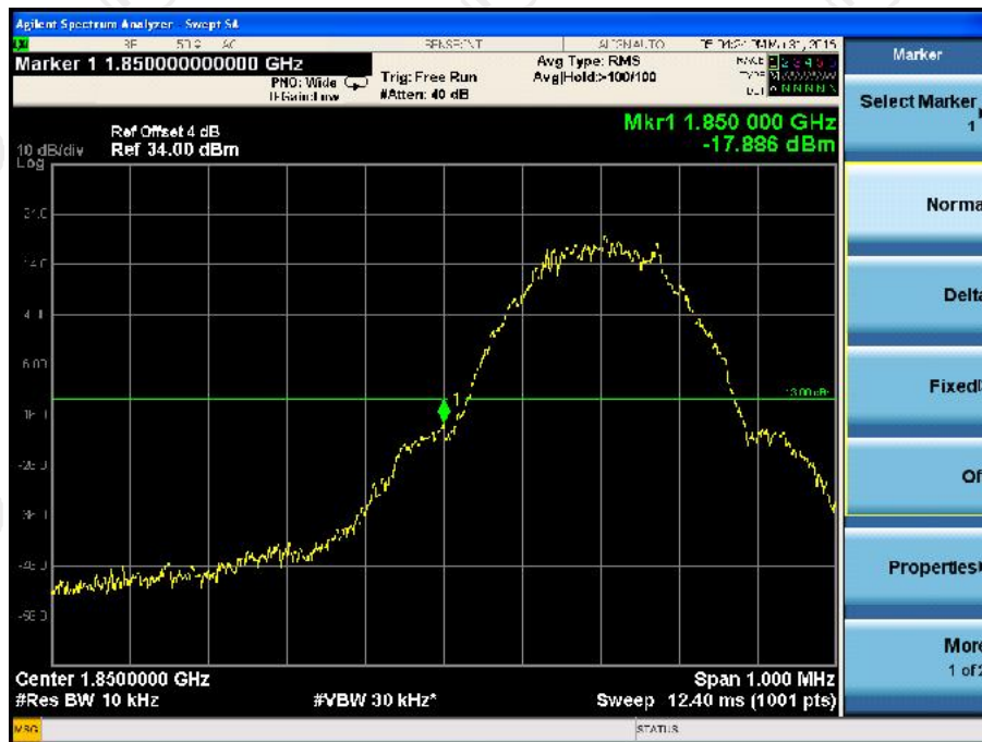
Higher Band Edge Plot on Channel 810
