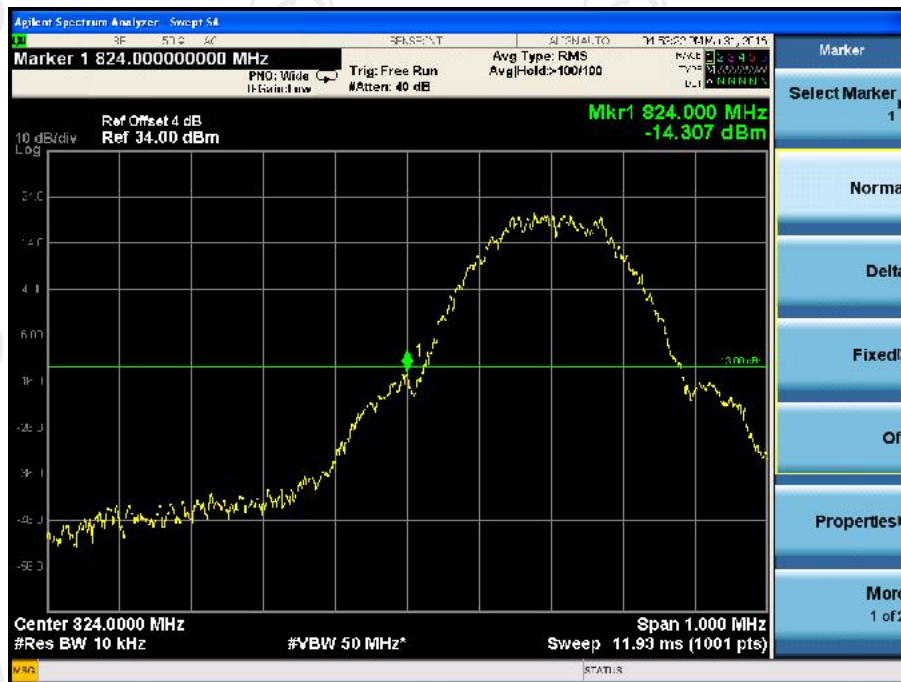
Higher Band Edge Plot on Channel 251
