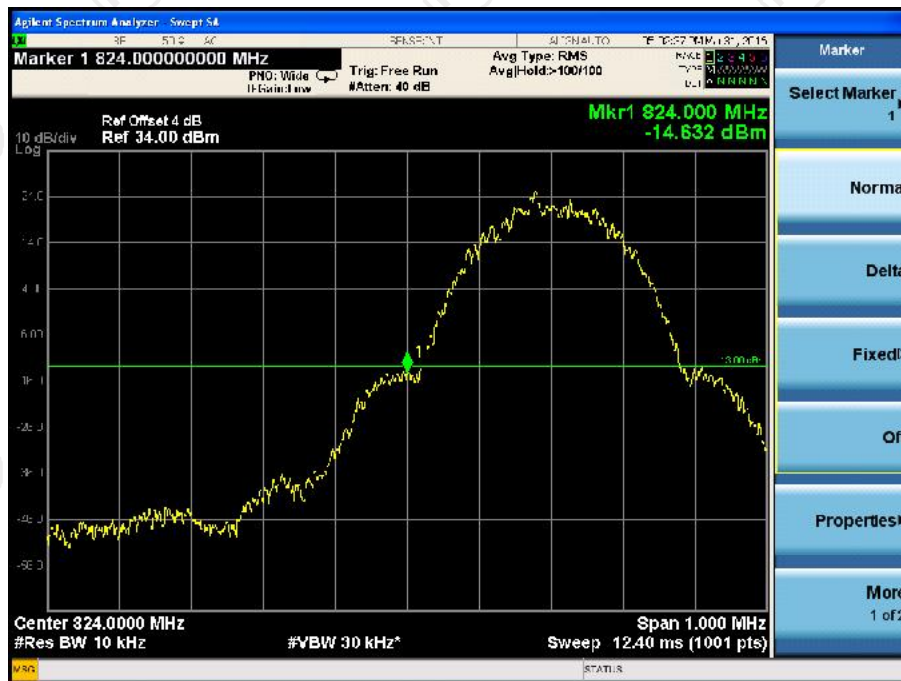
Higher Band Edge Plot on Channel 251
