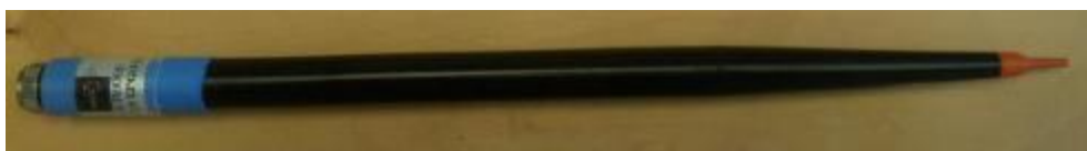
Figure 1 – MVG COMOSAR Dosimetric E-field Dipole
