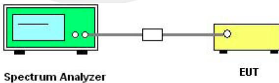
The EUT is coupled to the Spectrum Analyzer; the RF load attached to the EUT antenna terminal is 50Ohm; the path loss as the factor is calibrated to correct the reading. Make the measurement with the spectrum analyzer's resolution bandwidth(RBW) = 100 kHz. In order to make an accurate measurement, set the span greater than RBW.
