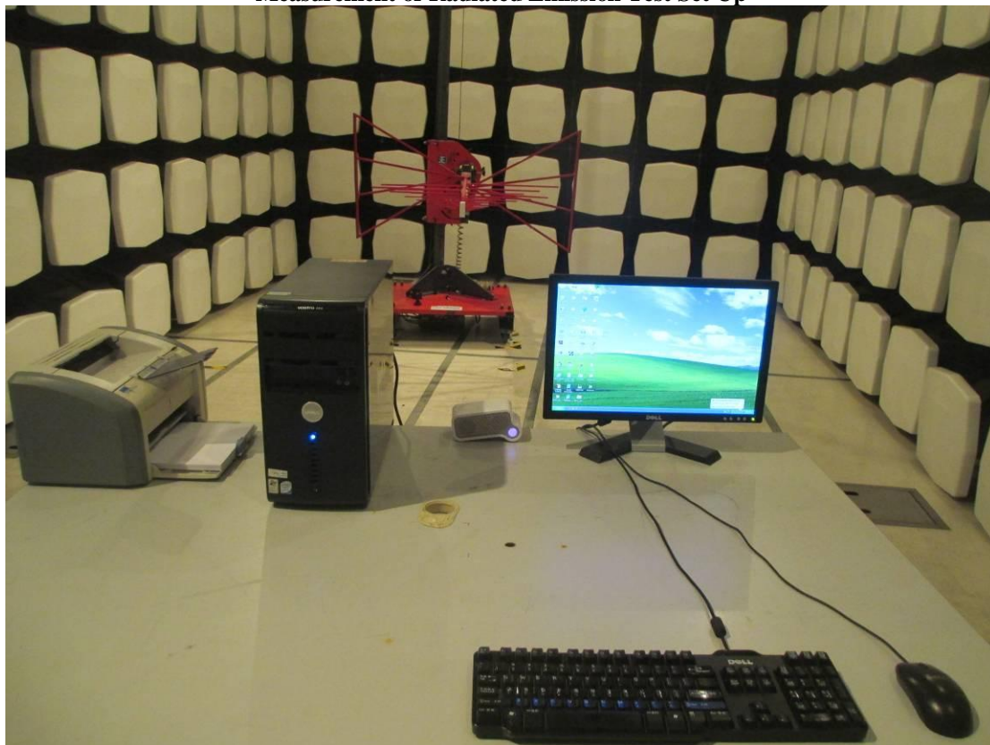
Measurement of Radiated Emission Test Set Up
