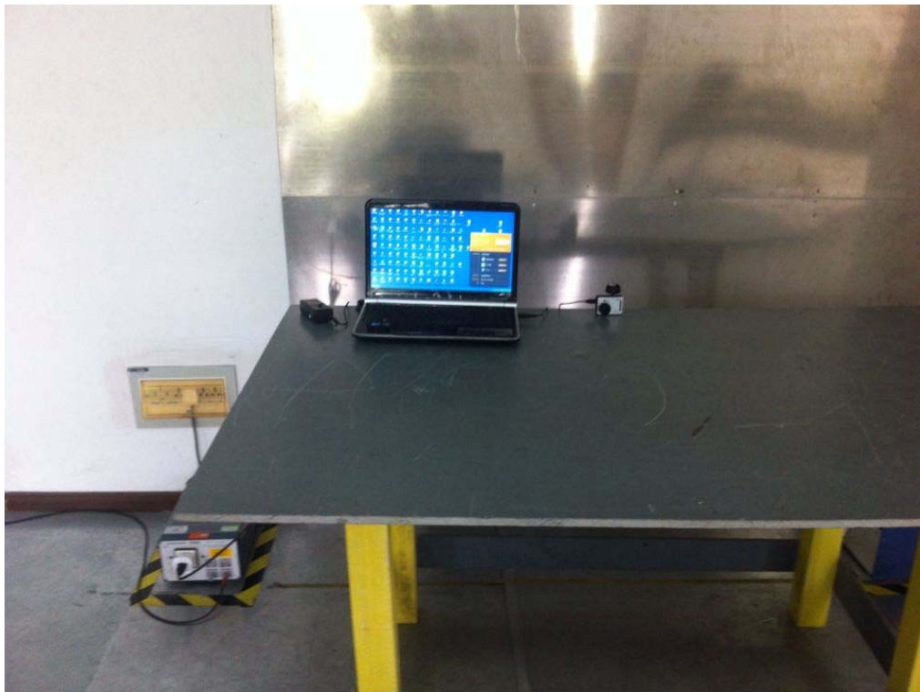
Conducted Emissions Test Setup Front View
