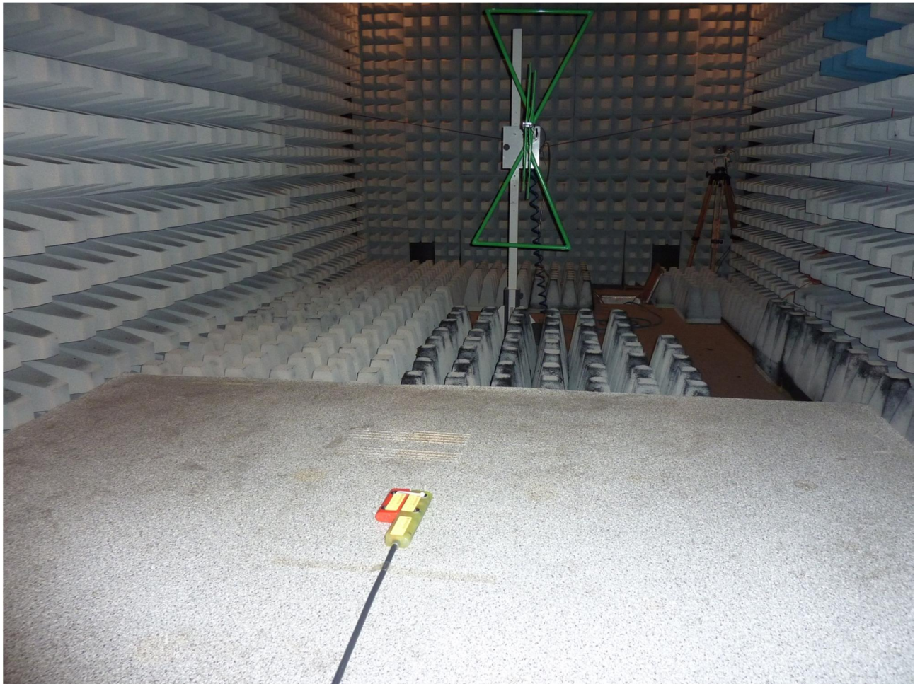
131297emi1.JPG: Test setup preliminary measurement (E-field)
