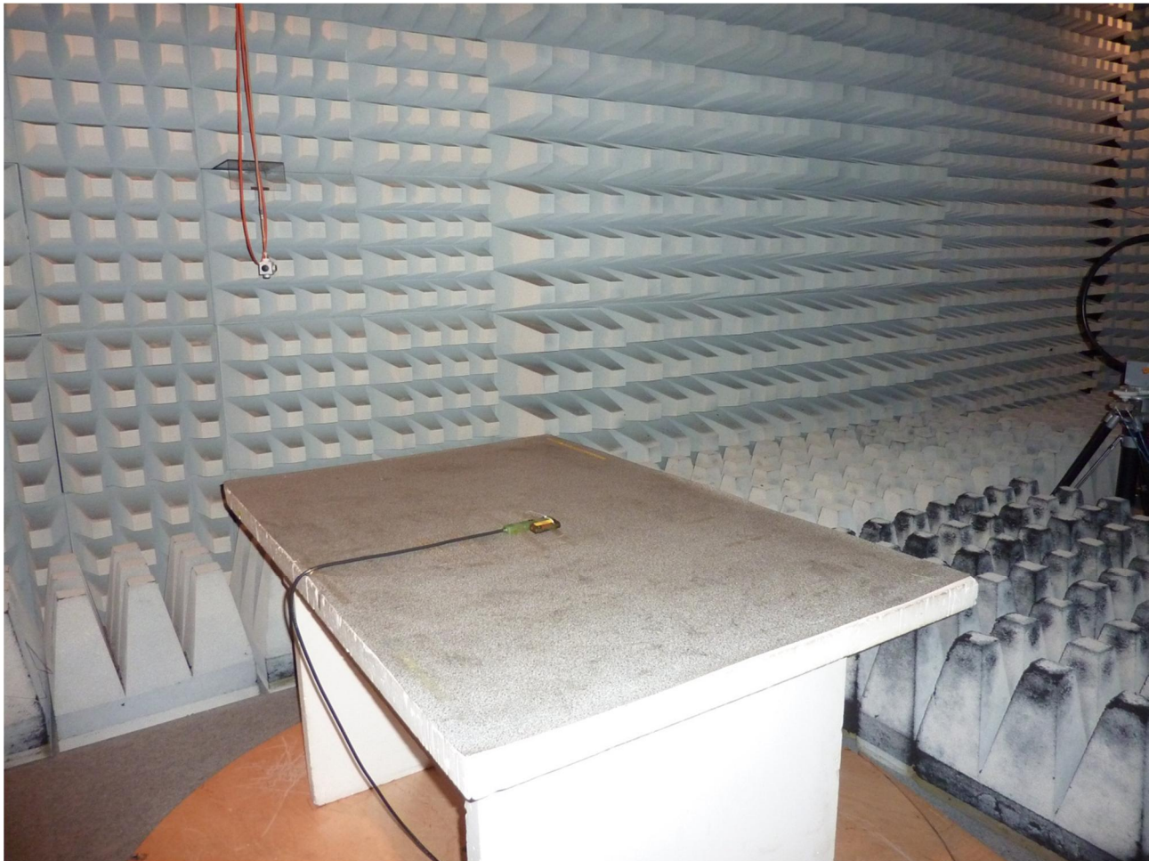
131297emi2.JPG: Test setup preliminary measurement (H-field)
