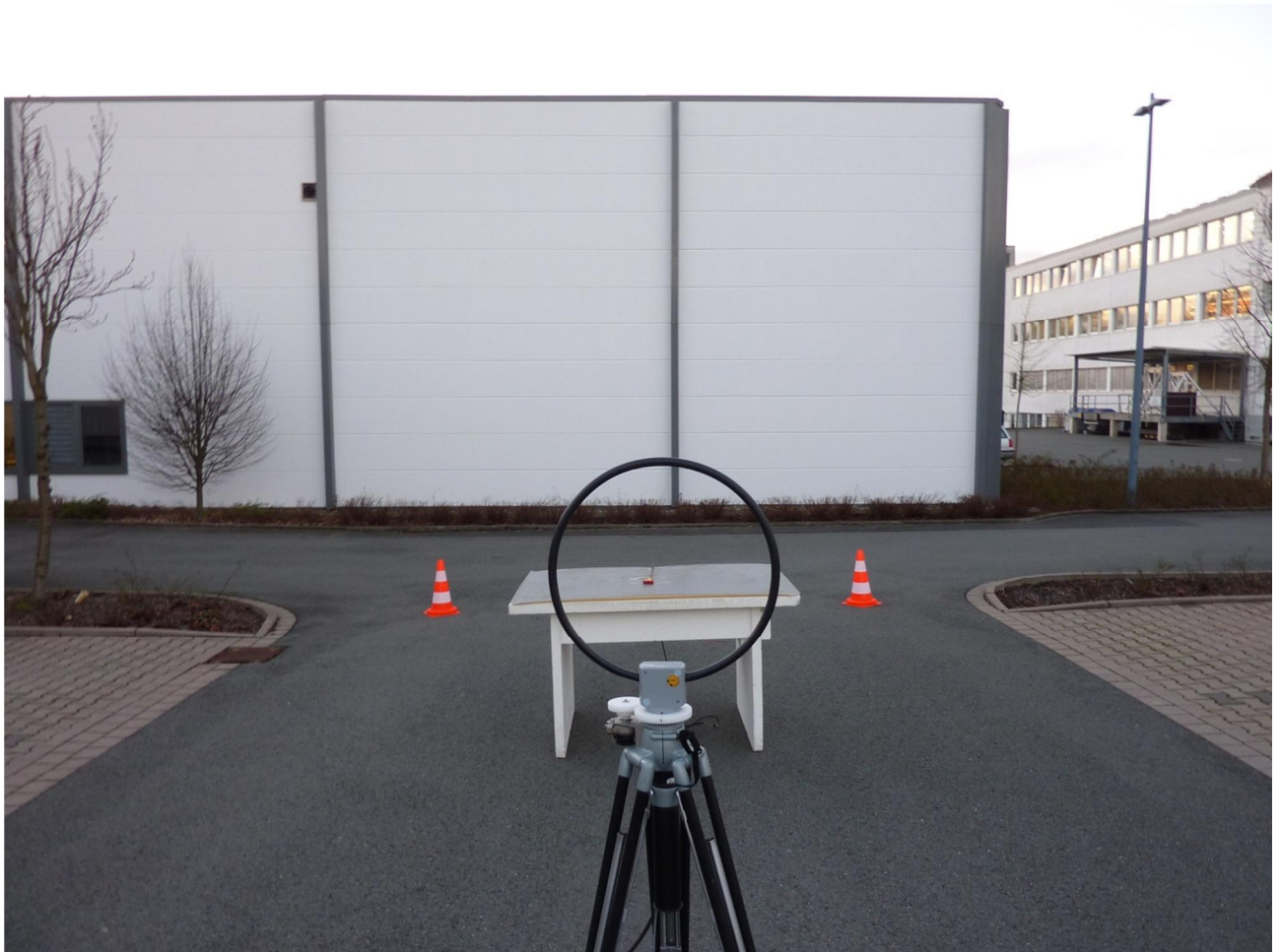
131297emi4.JPG: Test setup final measurement (H-field)
