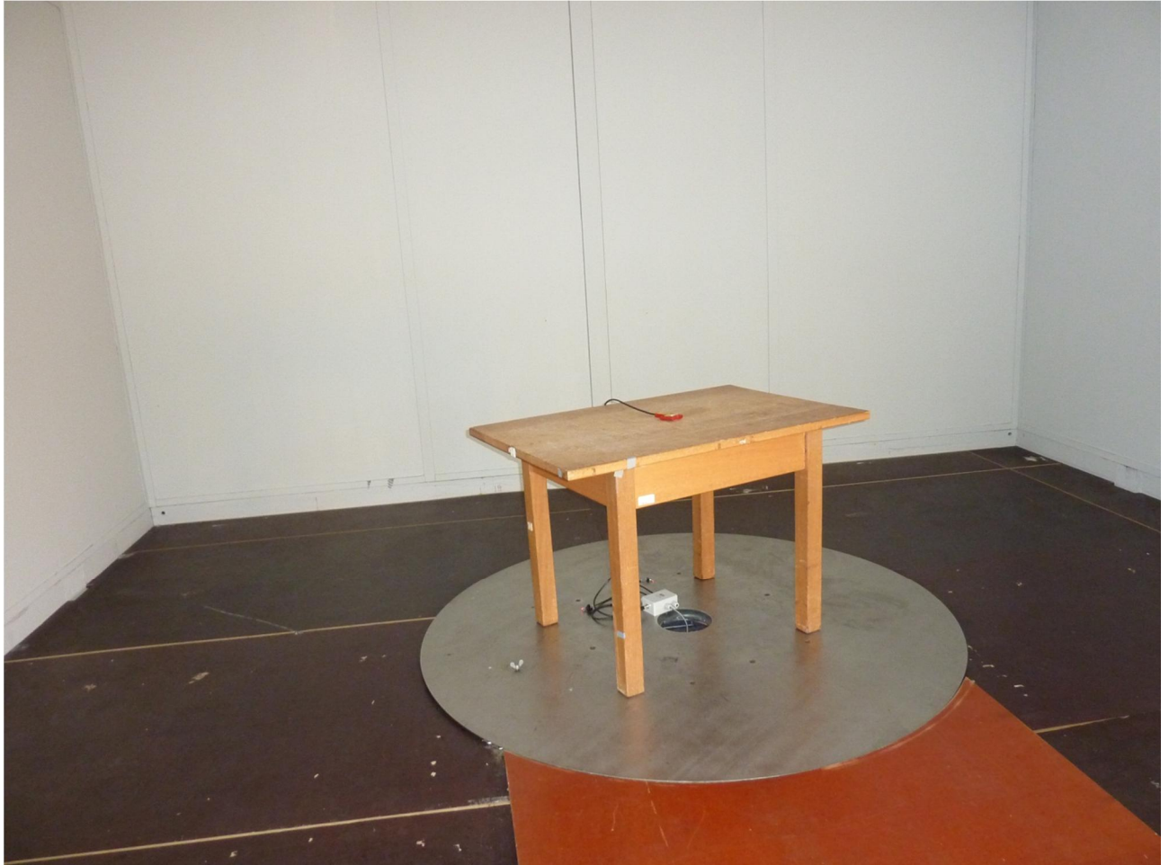
131297emi3.JPG: Test setup final measurement (E-field)
