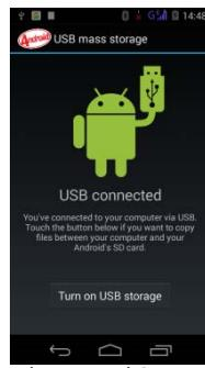
Then we mount the external SD card and internal memory as USB disk. And it is possible to manage your phone data directly on your computer. Once finished, click "Turn off USB storage" to release SD card from computer as following;
