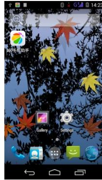
The status bar shows the time, signal strength, battery status, and notification.
