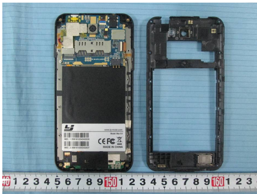
EUT – Cover off View
