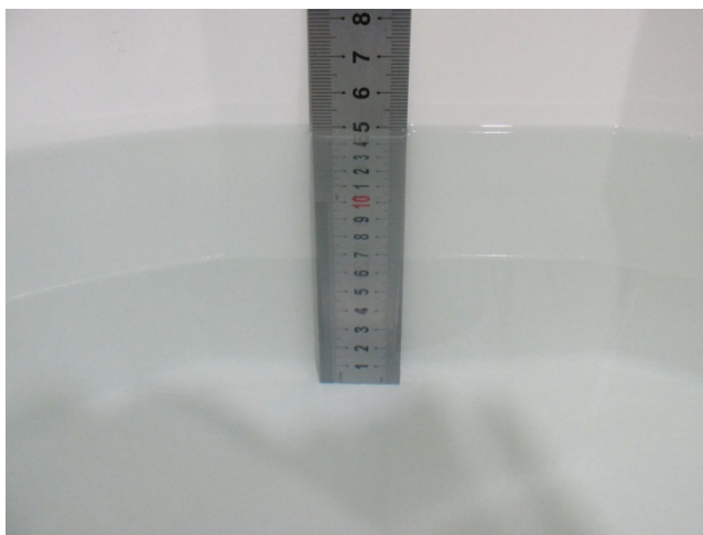
Fig.16 Body Liquid of 1800MHz(15cm)
