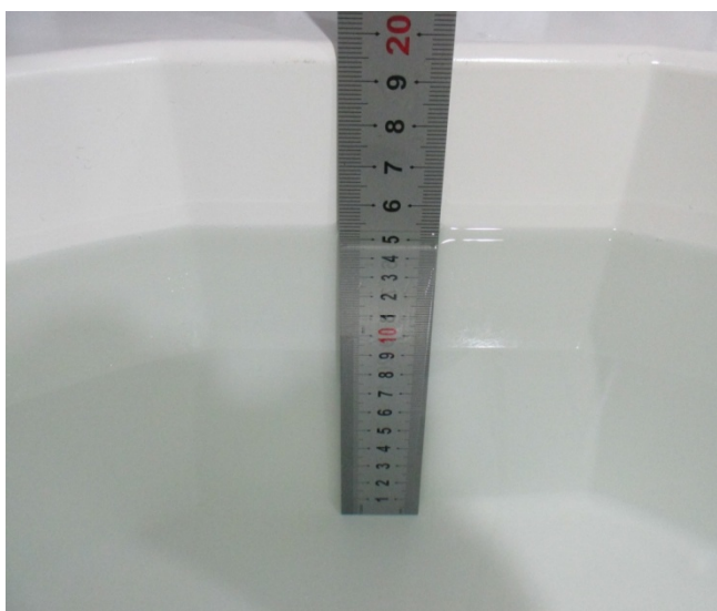
Fig.20 Body Liquid of 2450MHz(15cm)
