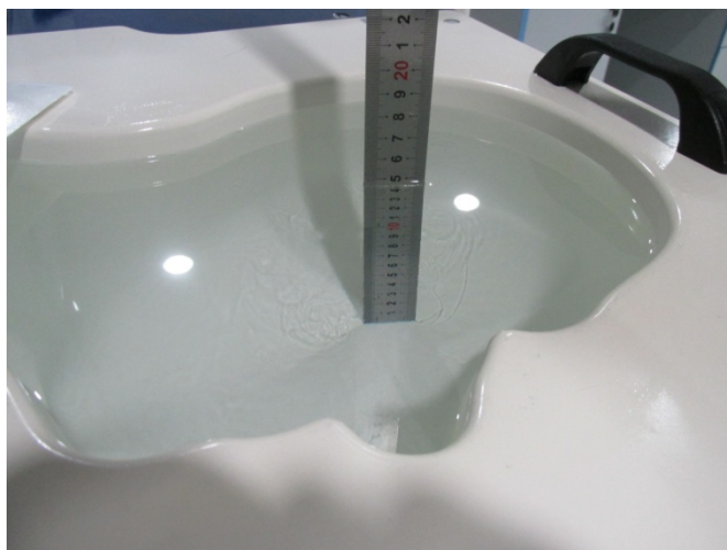
Fig.19 Head Liquid of 2450MHz(15cm)
