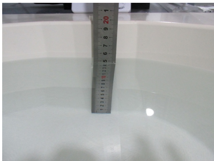
Fig.14 Body Liquid of 835MHz(15cm)
