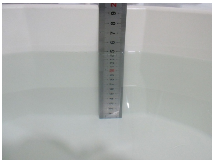
Fig.17 Head Liquid of 1900MHz(15cm)
