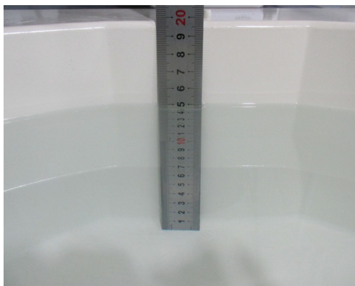
Fig.18 Body Liquid of 1900MHz(15cm)
