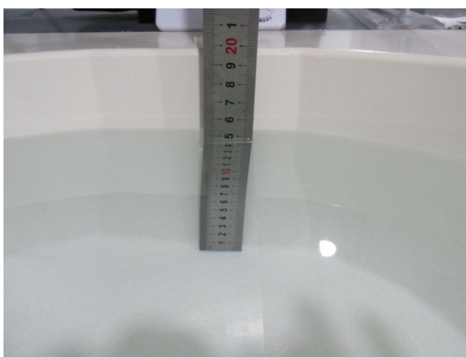
Fig.15 Body Liquid of 835MHz(15cm)
