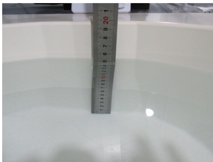
Fig.12 Body Liquid of 750MHz(15cm)
