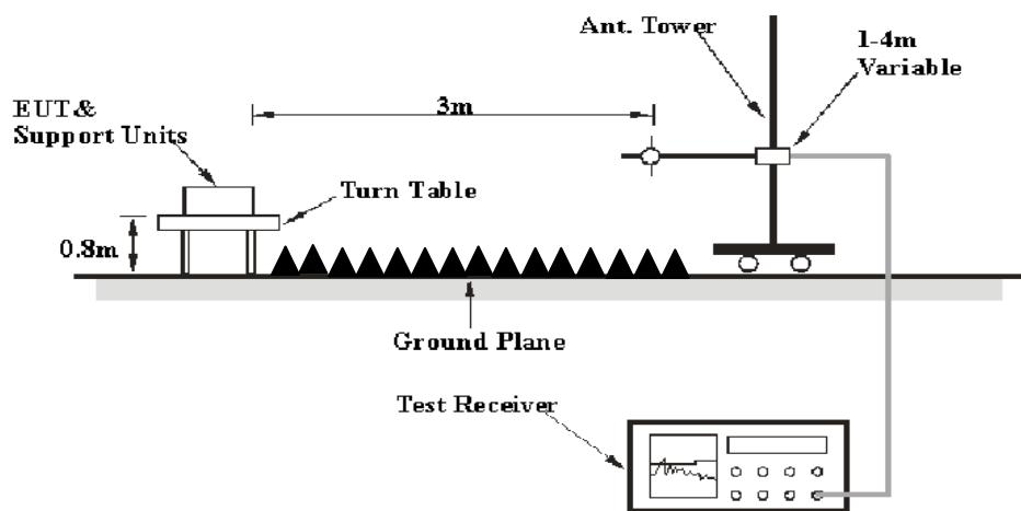
The radiated emission tests were performed in the 3 meters chamber test site, using the setup accordance with the ANSI C63.4-2009. The specification used was the FCC Part 15.109 Class B limits.
