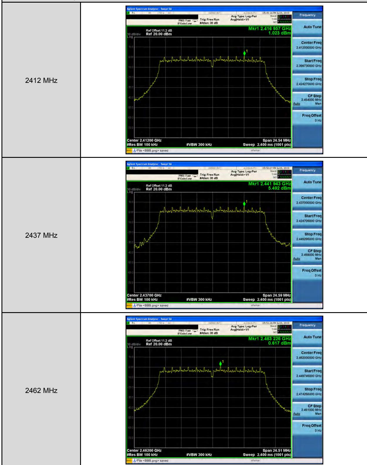
Mode 4: IEEE 802.11n 2.4 GHz 20 MHz Continuous TX mode \_ANT-0
