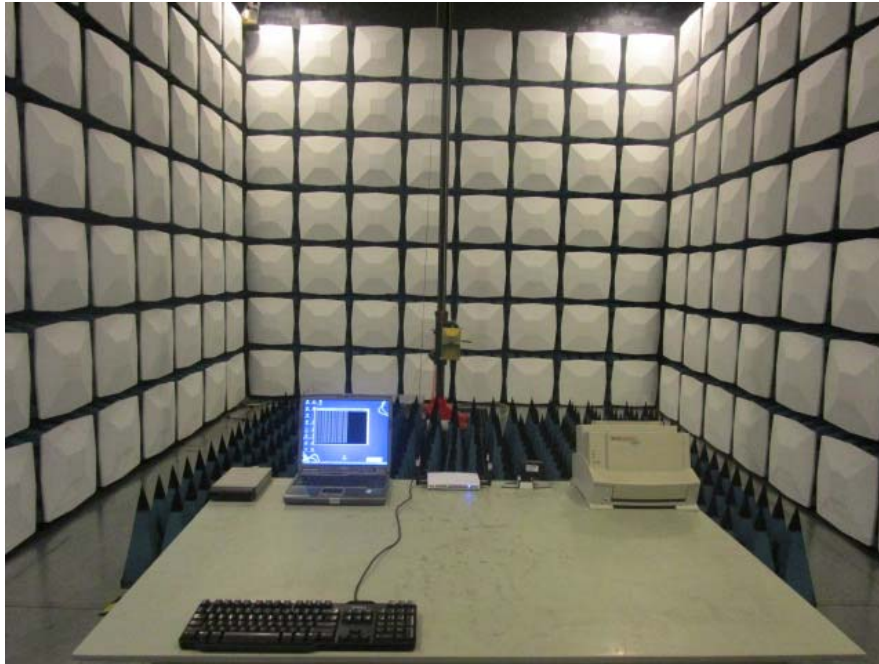
Radiated Emission –Front View (Above 1 GHz)
