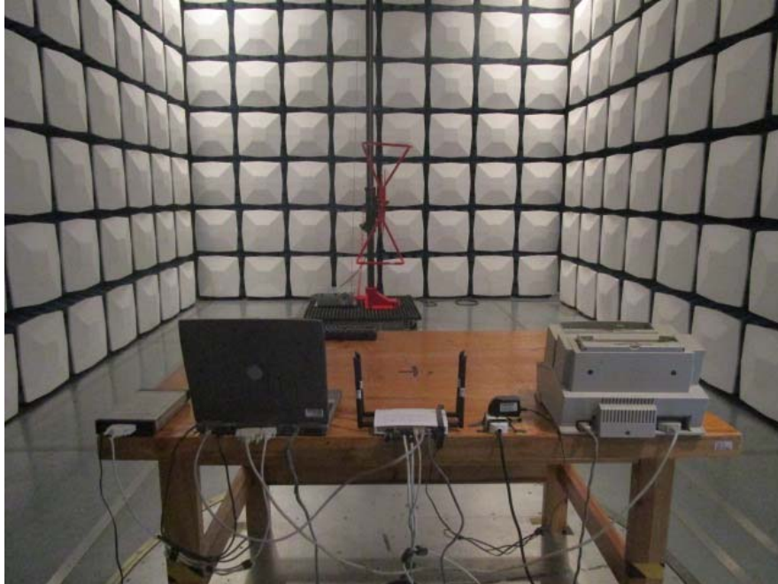
Radiated Emissions –Rear View (Below 1GHz)
