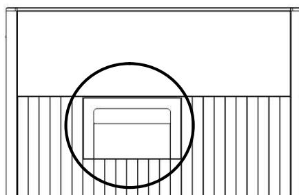
Remove the cover upward.
