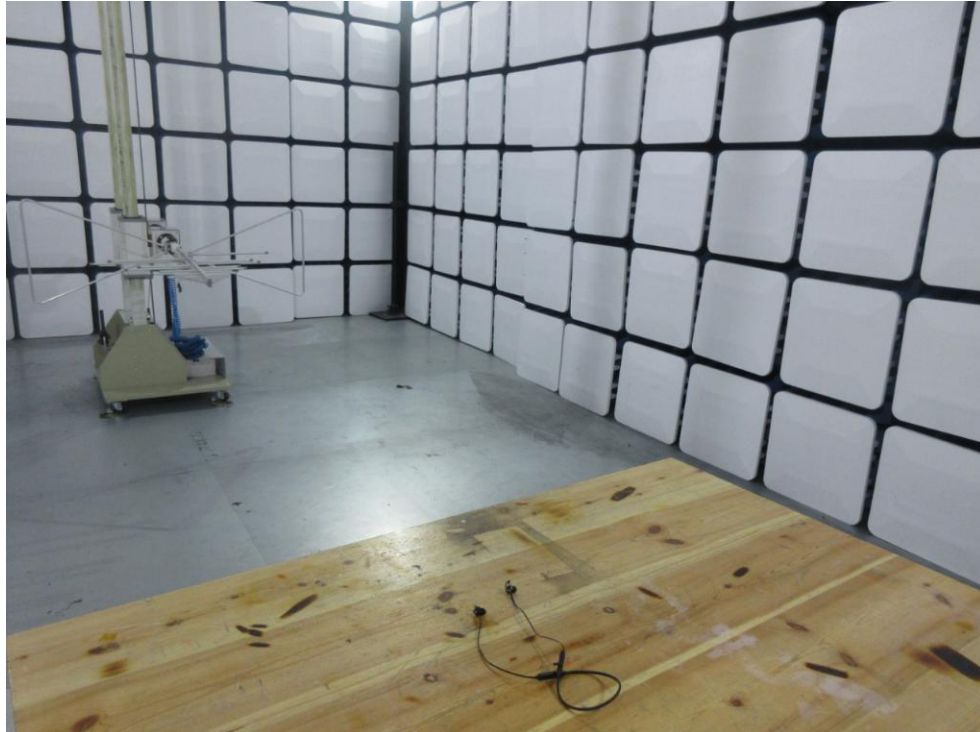
Photo of Radiation Emission Test
