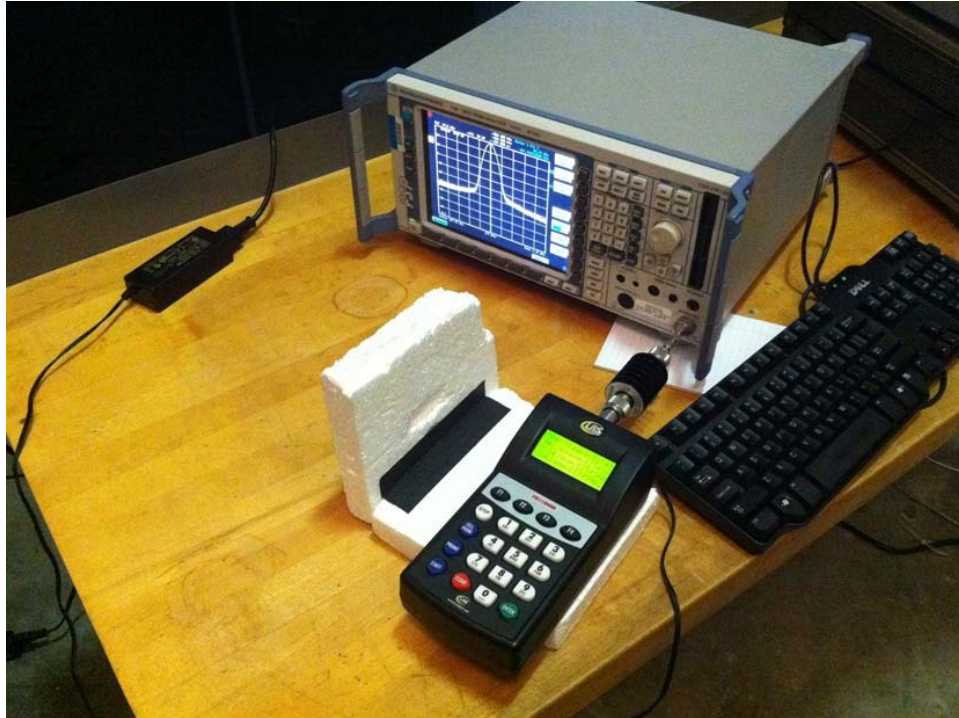
Conducted: Fundamental Power, Spurious, Bandwidth
