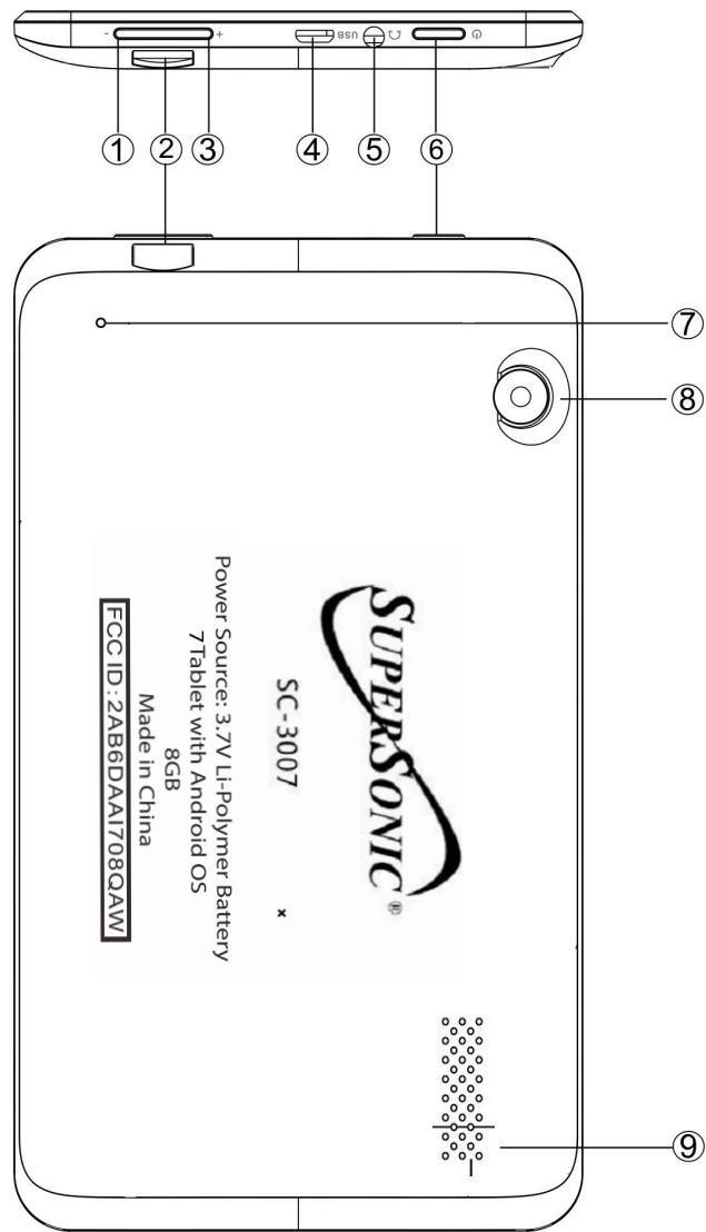
① VOL- key      ② Micro SD      ③ VOL+ key      ④ Micro USB OTG
