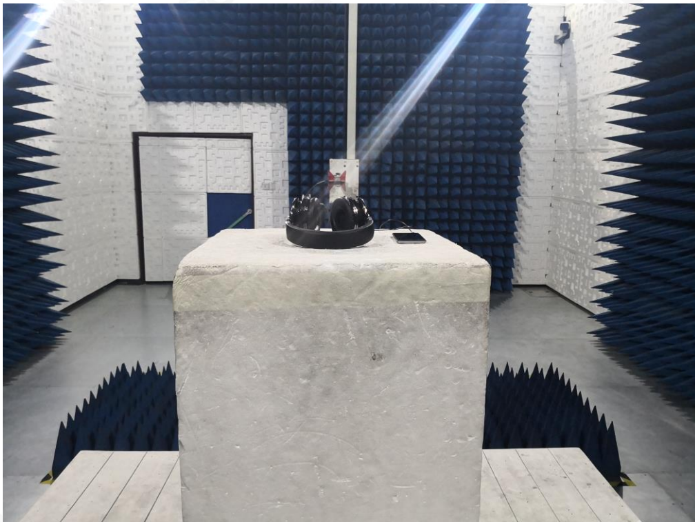
RADIATED EMISSION TEST SETUP ABOVE 1GHZ
