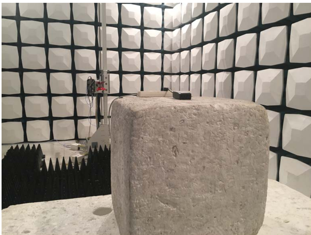
Description: Radiated Emission Test Setup for 1~18GHz
