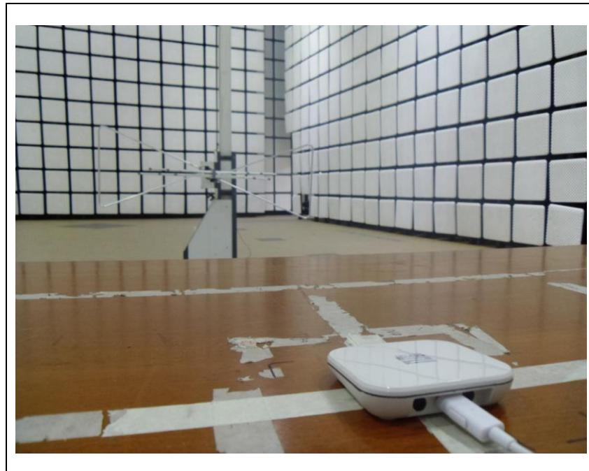
**B. Photo of Radiated Spurious Emission Test (Above 1 GHz)**
