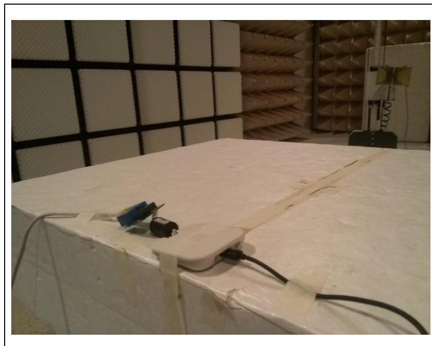
**C. Photo of Transmitter AC Power Line Conducted Emission Test**
