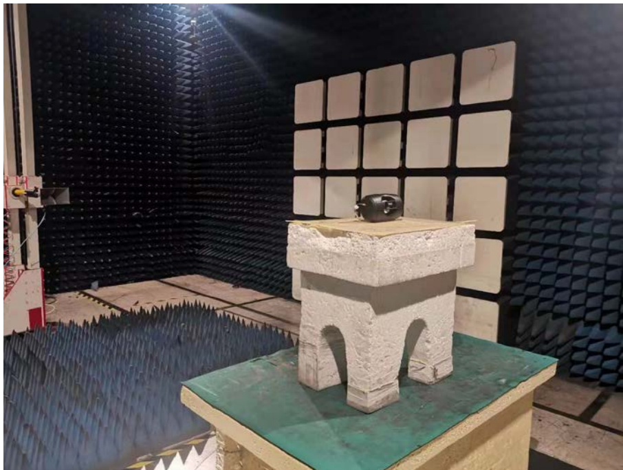
Spurious Emission Test Setup (Above 1GHz)
