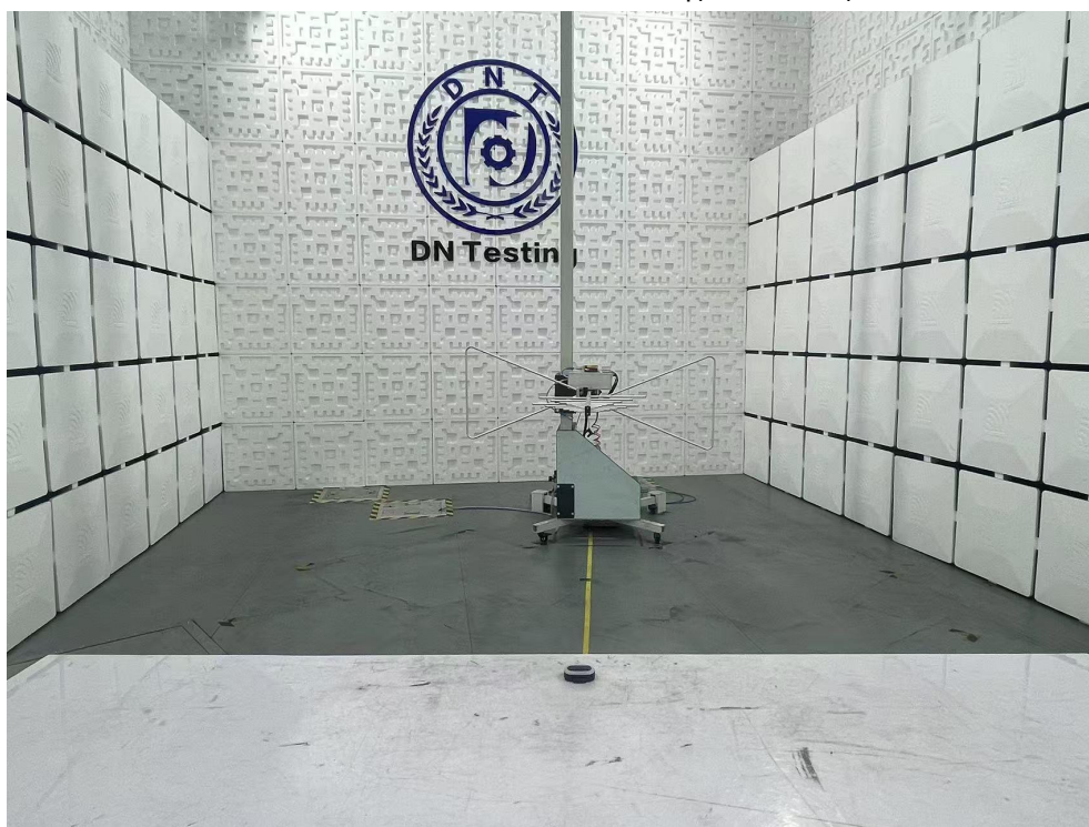
Radiated Emission Test View|(Below 1G)
