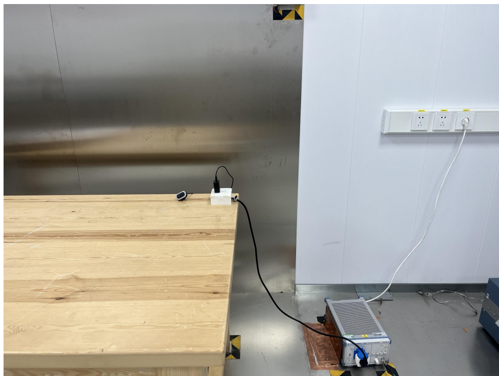
Radiated Emission Test View|(Below 1G)
