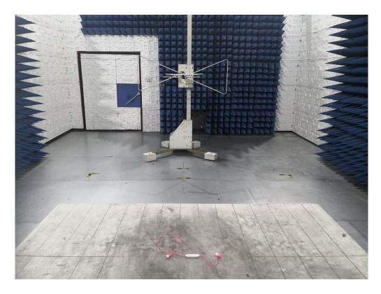
RADIATED EMISSION TEST SETUP ABOVE 1GHZ
