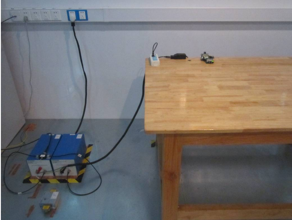
Conducted Emissions Test Setup Front View
