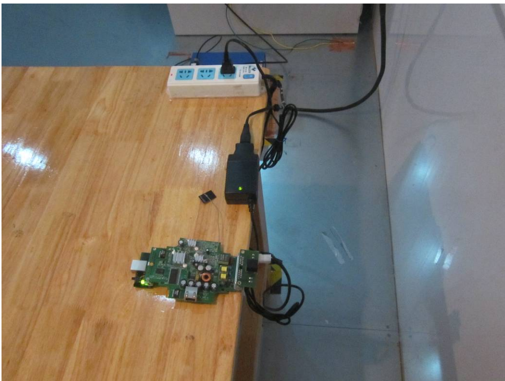
Conducted Emissions Test Setup Side View
