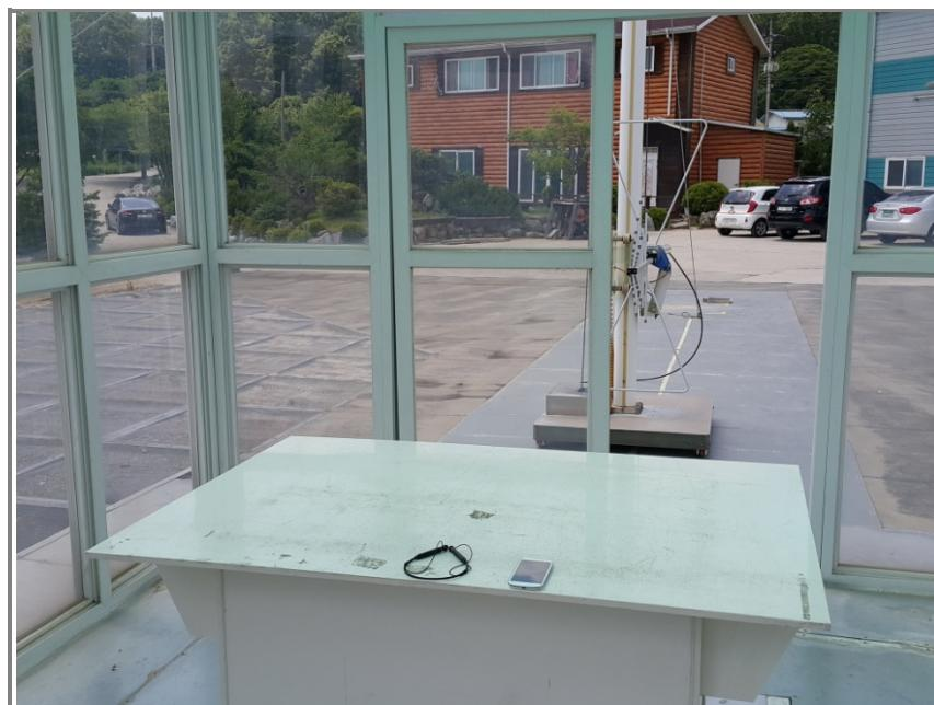
**Photo of radiated spurious emission at above 1 000 MHz**
