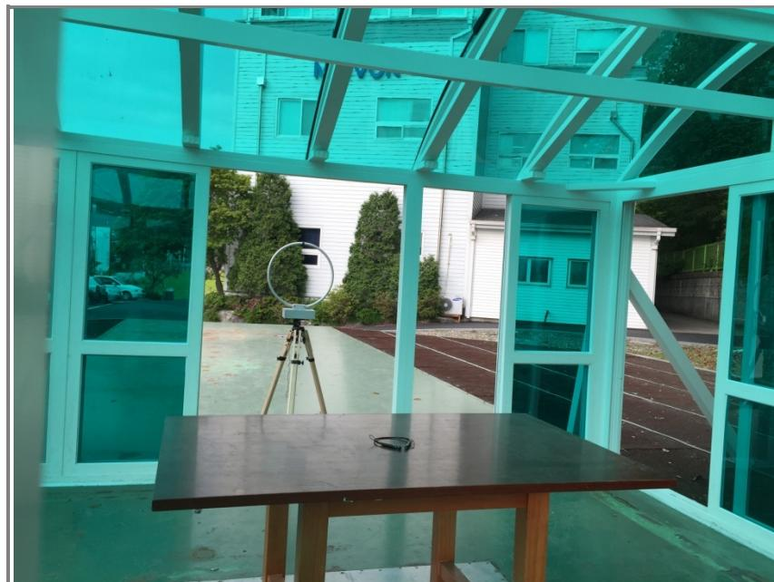
**Photo of radiated spurious emission at 30 MHz ~ 1 000 MHz**
