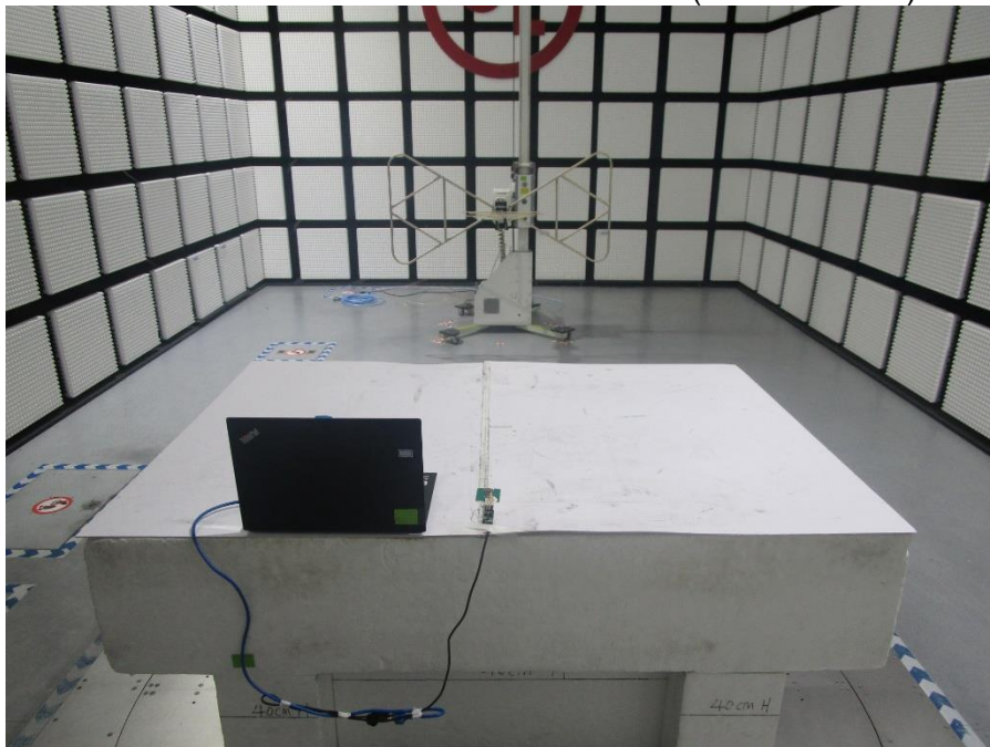
RADIATED RF MEASUREMENT SETUP (Below 30MHz)
