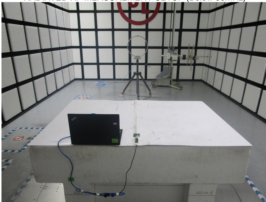
RADIATED RF MEASUREMENT SETUP (Below 30MHz)
