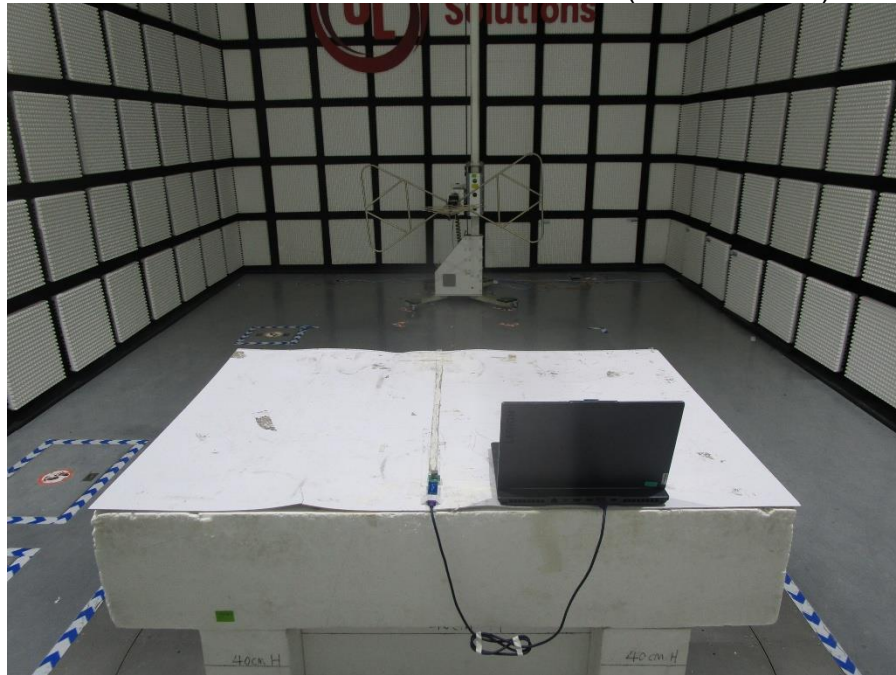
RADIATED RF MEASUREMENT SETUP (30MHz~1GHz)
