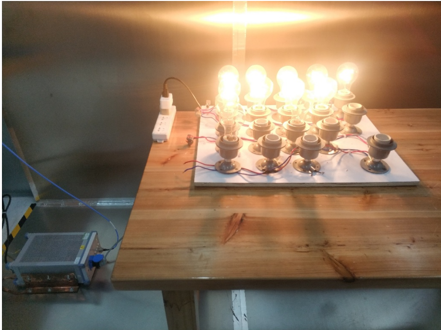
Photograph 3: Set-up for Conducted Emissions
