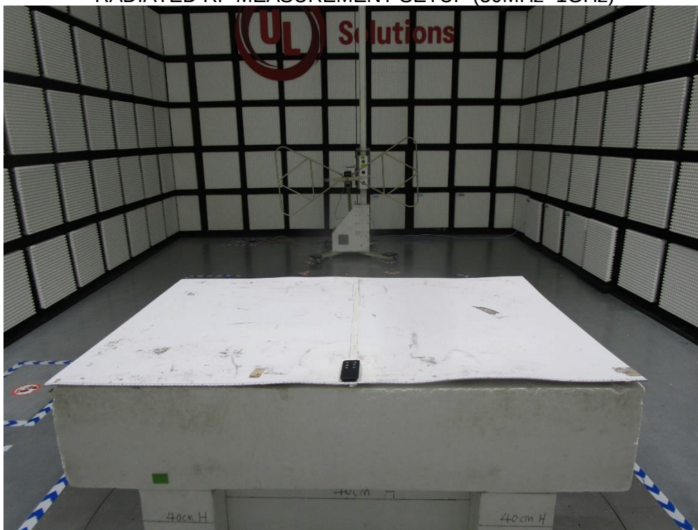
RADIATED RF MEASUREMENT SETUP (30MHz~1GHz)
