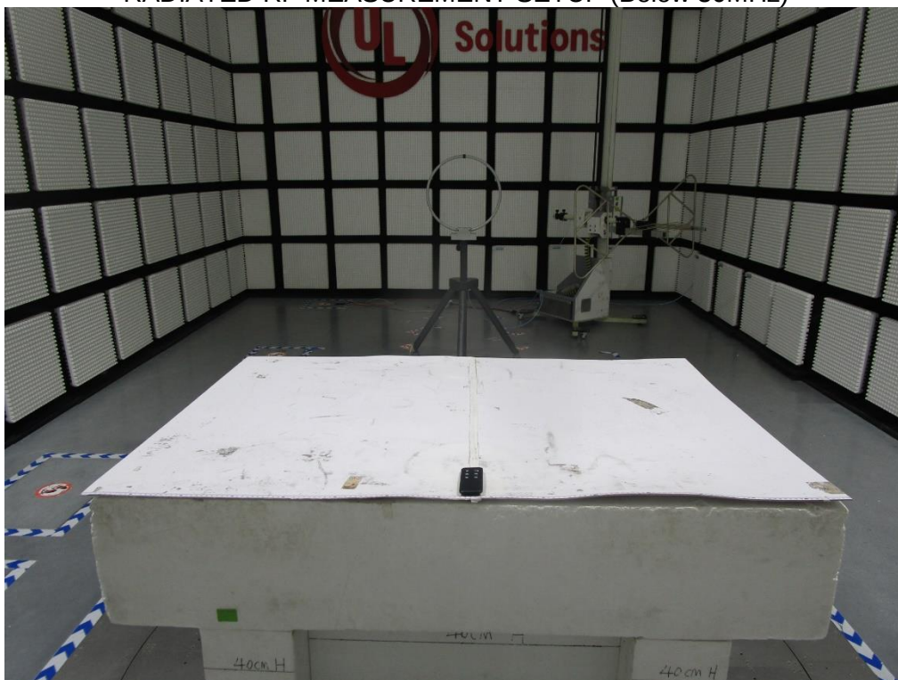
RADIATED RF MEASUREMENT SETUP (Below 30MHz)
