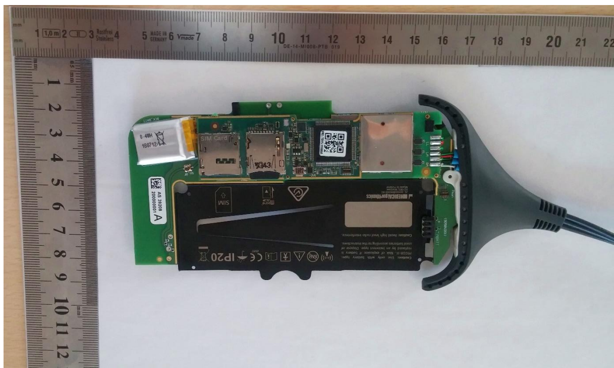
Fig.2 P4TR-AA-ADS (bottom view without screen and enclosure )
