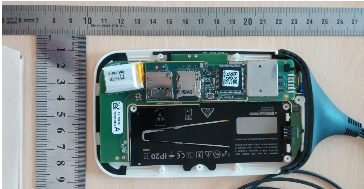
Fig.1 P4TR-AA-ADS (bottom view without bottom enclosure)
