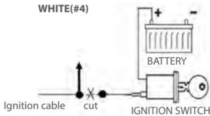
**Note :** If the ignition switch has three terminals, the installation is not valid for this system.
