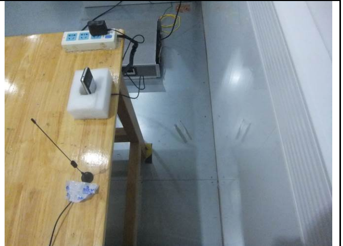
Conducted Emissions Test Setup Side View
