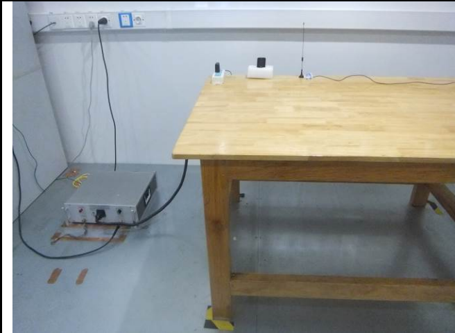
Conducted Emissions Test Setup Front View
