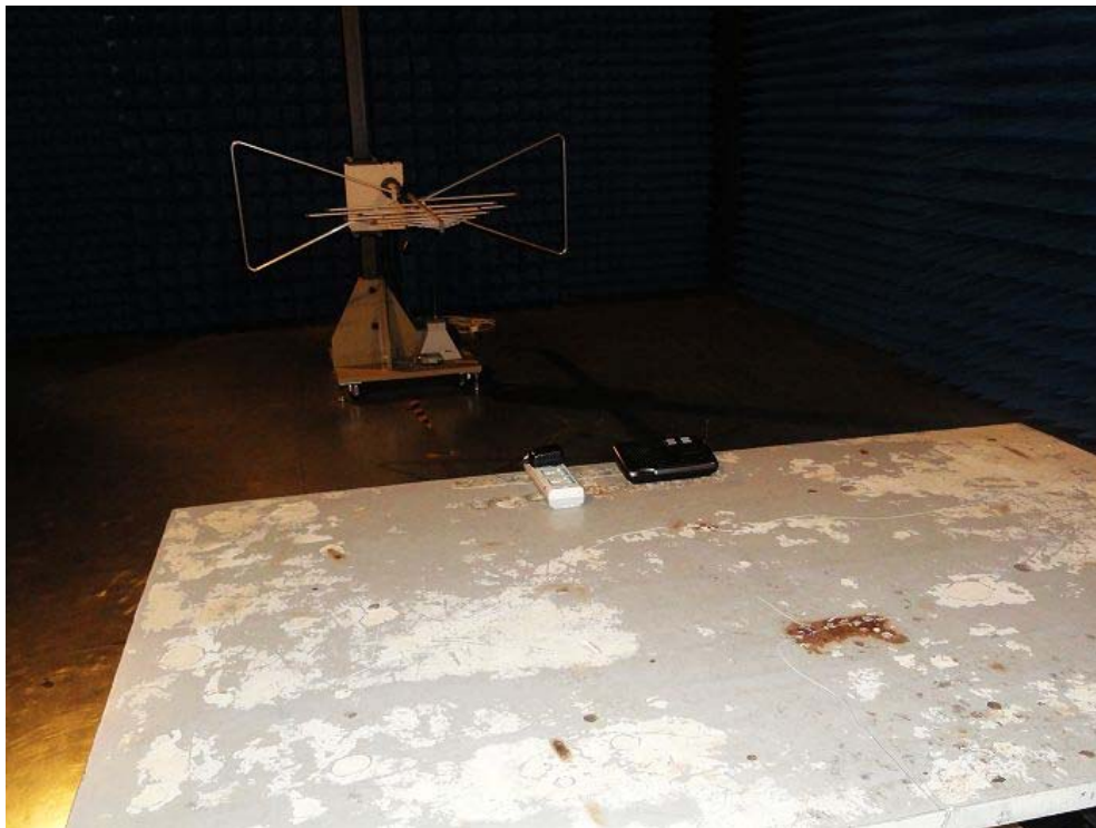
Radiated emission test view
